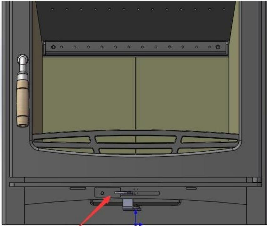
**This is 18mm stop plate, we could take off or reverse placing when we need standard version.**
